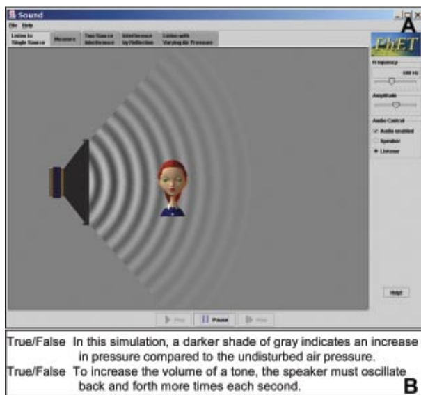
Fig. 7. In the Sound sim (Panel A), a speaker oscillates back and forth producing pressure waves that propagate from the speaker. Students can: adjust frequency and amplitude; see changes in the pressure waves and hear changes in pitch and volume; use a ruler and timer to measure speed, frequency, period, and wavelength; and look at and listen to the interference of waves from two speakers. In Panel B, true/false questions guide students' exploration.
